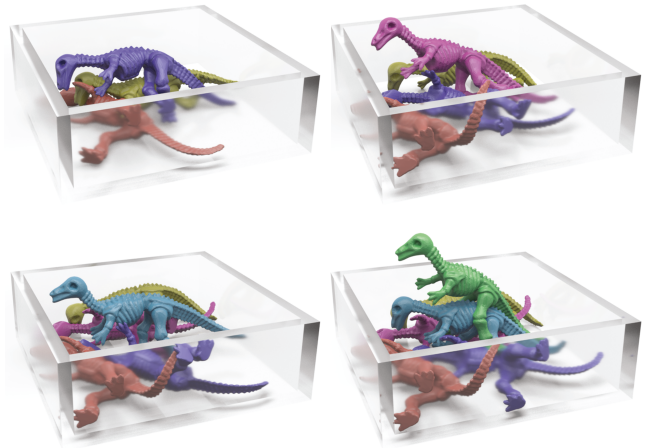
Fig. 15. Real-time simulation of six falling dinosaur models using modal derivative (30 modes for each dinosaur). The first-order derivative modes are computed using CSFD, and we use Fung, Mooney-Rivlin, Ogden, Yeoh, Arruda-Boyce and Polynomial materials for each dinosaur.
