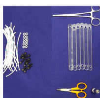
Figure 1. Assembling a tensegrity mechanism - 1) Perforated rigid links allow variable points of connection and nut-bolt combinations act as adjustable clamps. 2) Links are aligned on a planar surface and interconnected using oversized cables. 3) The cables are individually tensioned, without need of external jigs, 4) to construct the final balanced tensegrity mechanism.
