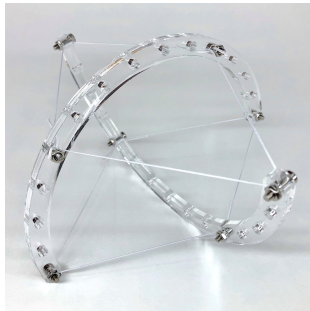
(3c) Dual-axis wobble locomotion of two curve-link mechanism.
