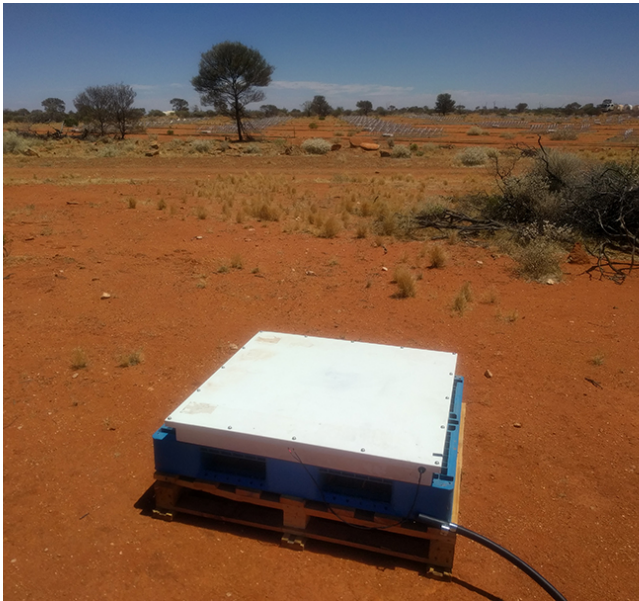
Figure 9. The prototype SKAPA cosmic ray detector (white box) deployed near the MWA core at the MRO. It is raised off the ground with pallets to avoid surface water. Power and data return are enclosed via the black cable housing. The detector has been tested to ensure compliance with MRO RFI requirements, and has been detecting cosmic ray muons since its deployment in October 2018. Photo credit: Justin Bray.
