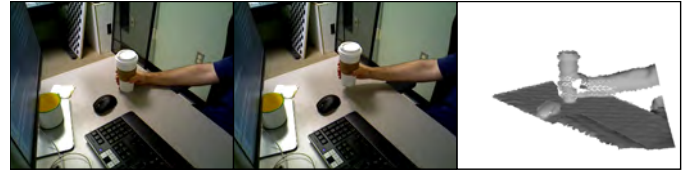
(a) Left, middle: color frames (source and target) captured by an RGB-D camera. Right: warped source frame by the result of a standard non-rigid registration algorithm.
