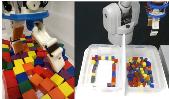
Fig. 6. (Left) Inserting a finger into the bottom layer of bin is difficult as there are few gaps for insertion. (Right) Blocks around the perimeter of the left start container are not transferred during the untimed task as a grasp plan was difficult to find.
