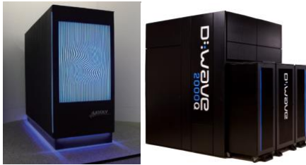
Fig. 13. Annealing machines for Ising combinatorial optimization. Left: CIM-based LASOLV from NTT. Right: D-Wave Systems 2000Q based on quantum annealing.
