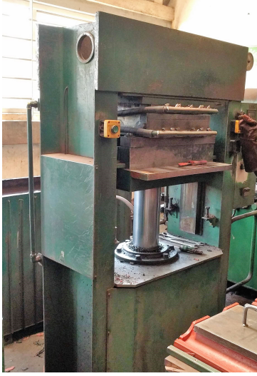
FIGURE 5. Photo of Tile Forming Press used at Resintile
