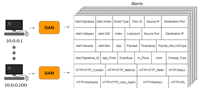
Fig. 1: Individual GAN models may be used to synthesize alerts based off Target IP and historical data.
