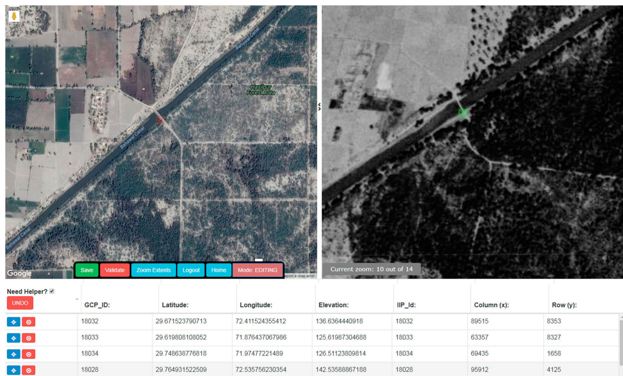
Figure 5. A screen shot of Sunspot, an online CORONA imagery orthorectification tool developed by the CORONA Atlas Project.
