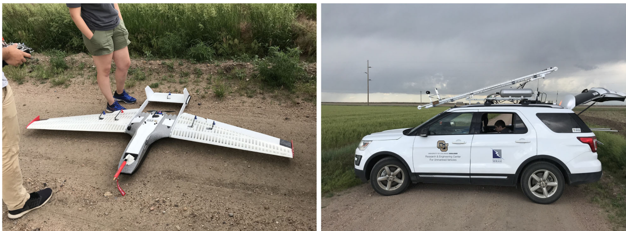
FIGURE 4 Left: The RAAVEN unmanned aircraft waiting for flight control systems to initialize. Right: Tracker 1 with the RAPCAT configured for launch. During nomadic operations, the RAAVEN undergoes preflight checks while sitting on the two posts extending from the back of the Tracker [Color figure can be viewed at wileyonlinelibrary.com ]
