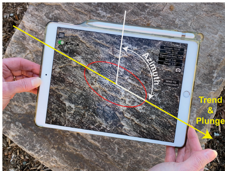
Figure 3. Using the edge fabric tool. The mobile device is held parallel to the plane being photographed. The app calculates the edge fabric ellipse and reports its azimuth (long axis of the ellipse, relative to “up” on the screen), its trend and plunge in space, and its axial ratio E . Calculations take 5 seconds or less. The analysis can be captured as a screenshot, and the trend and plunge can be copied for pasting into Stereonet Mobile (Allmendinger, 2019). StraboTools locks to landscape display.
