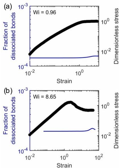
FIG. 5. Typical result from start-up to steady shear experiments showing the change in the fraction of dissociated bonds  $f_d$  and dimensionless stress  $\tilde{\sigma}$  as a function of strain for two shear rates, (a)  $Wi = 0.96$  and (b)  $Wi = 8.65$ , where  $Wi = \gamma\dot{\gamma}\tau_r$ .
