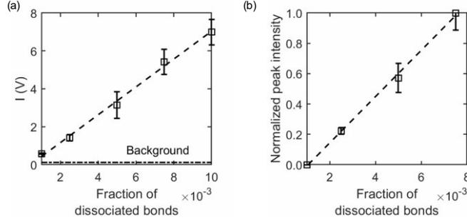
FIG. 3. (a) The calibration curve for calculating the fraction of dissociated bond from the measured photodetector output, obtained using standard solutions of known concentrations of terpyridine, at a gap height of 0.3 mm. (b) The fluorescence of the standard solutions was also measured on a fluorimeter, which supports the linear relation between the measured signal and the concentration.
