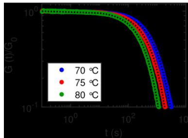
FIG. 7. Normalized stress relaxation following a small step strain (strain = 1%) at 70, 75 and 80 °C for the terpy-acrylamide gel. The dotted lines are fits to a phenomenological Kohlrausch-Williams-Watts (KWW) function.
