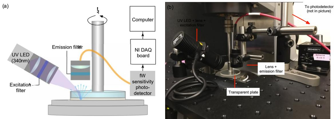
FIG. 2. Schematic and photo of the rheo-fluorescence set-up showing the position of the excitation source and collection lens, relative to the transparent upper plate.
