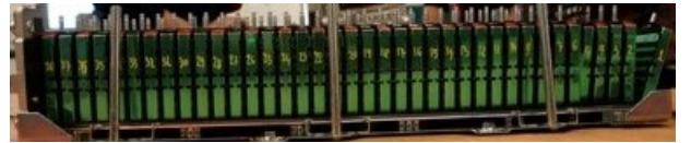
Fig. 3: Battery module with closely stacked cells
