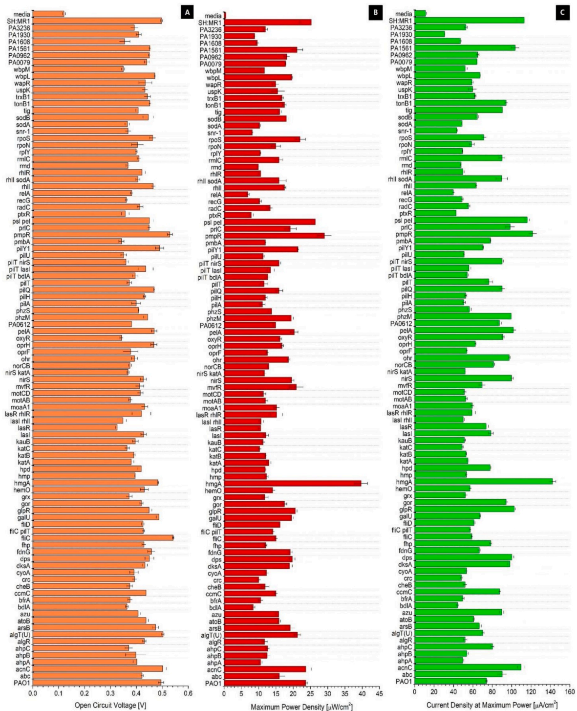
Fig. 5. (A) OCV, (B) maximum power density, and (C) current density at the maximum power are obtained from the polarization and power curves by the high-throughput parallel analysis on the array. The power and current outputs are normalized to the projected anode surface area.
