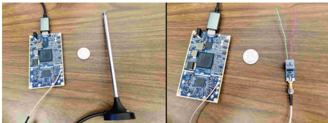
Fig. 18. Two antennas that have been used in RADAR. In both figures, the used LimeSDR is also shown.
