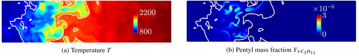
Fig. 9. Two-dimensional slices showing isocontours for the turbulent case ( \Delta t = 10^{-8} s). Two temperature isolines are superimposed in white ( T = 1000 K and T = 1900 K).
