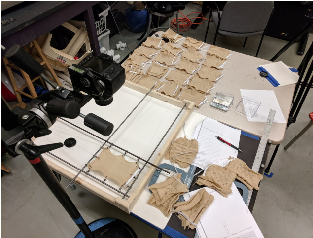
Figure 6: Data set measurement setup, including camera, scale, and stretching rig.
