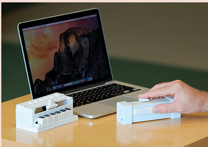
Figure 3. A tangible scrollbar and task switcher. 2
