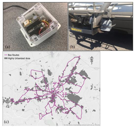
Fig. 1. Vehicle-borne sensor system, (a) Vehicle-borne sensor, (b) sensor mounted on bus, (c) bus routes in Athens, GA with highly urbanized areas such as malls, shoping plazas, urban core are combinmedly highlighted in dark gray.
