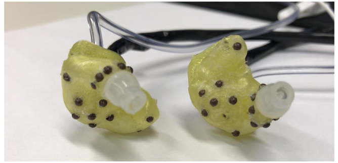
Fig. 1. The earpieces fabricated from 3D CAD models of the subject's ear shown here embedded with 17 Ag-Ag/Cl electrodes each. A air tube comes through the lumen of the earpieces the provide sound directly the ear canal.
