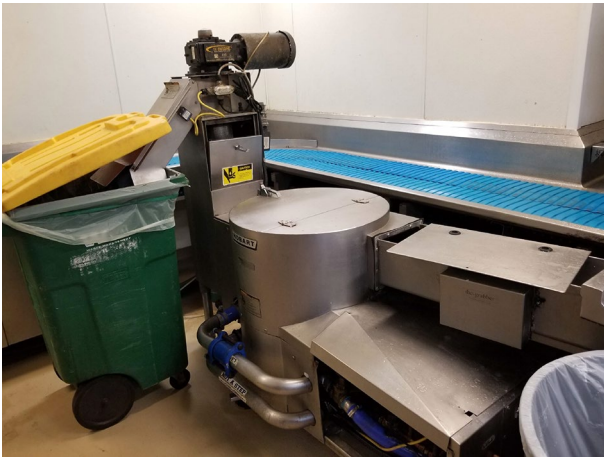
Fig. 3 Example of interacting decentralized and centralized waste management systems: an urban university cafeteria using a food waste pulper to remove water (and associated weight) from food waste to minimize cost and impacts of hauling residual wastes to a rural anaerobic digester. Photographed by Callie Babbitt
