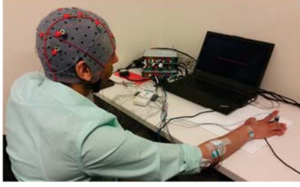
Fig. 1: Experimental Setup. The participant is tapping the texture mounted on the force transducer.
