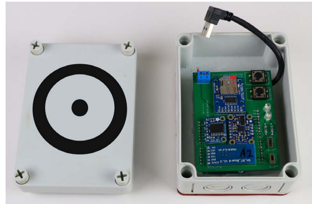
Fig. 4 Microcontroller setup composed of a custom PCB and sensors that tracked motion of the handle while researchers incremented users with a remote control
