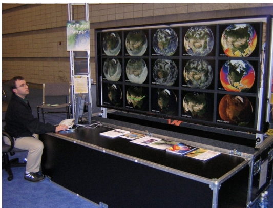
Figure 10: Picture of a portable SAGE wall that ships entirely within a road case. (Designed by collaborators at Calit2-Qualcomm Institute at UC San Diego.)
