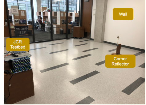
Fig. 3. Experimental setup for radar channel measurement using our mmWave JCR testbed.
