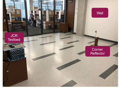
Fig. 4. Experimental setup to demonstrate SIMO feasibility.
