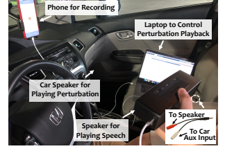
Figure 8: Illustration of the inside-vehicle setup.
