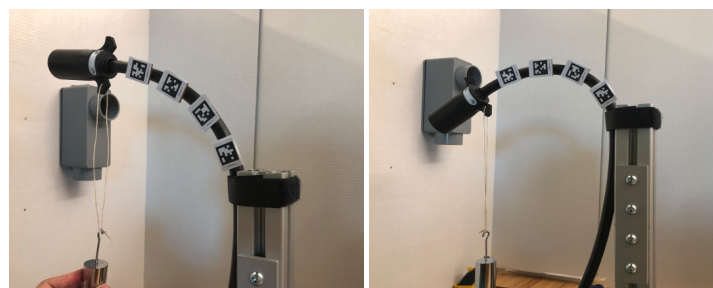
(a) Using apriltag to record the joint positions—start point (b) Using apriltag to record the joint positions—end point
