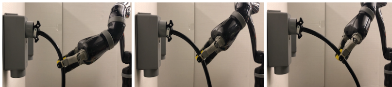
Figure 19. Experiment 1: The robot successfully grasps the cable with three different initial states.
