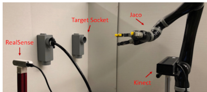
Figure 1. DARPA Robotics Challenge (DRC) Plug Task setup (© 2020 IEEE [29]).
