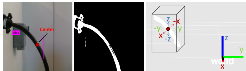
Figure 3. Steps for obtaining the filtered point cloud (© 2020 IEEE [29]): (left) YOLO object detection, (middle) color detection, (right) point cloud filter.
