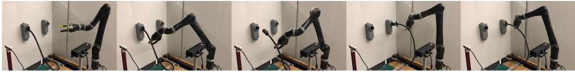
Figure 17. From left to right: The Jaco v2 robot completing the DRC Plug Task in the real world.
