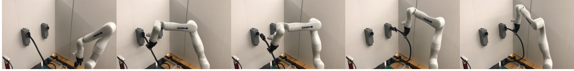
Figure 18. From left to right: The Gen3 robot completing the DRC Plug Task in the real world.
