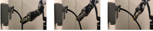
Fig. 10: Experiment 1: The robot successfully grasps the cable with three different initial states.
