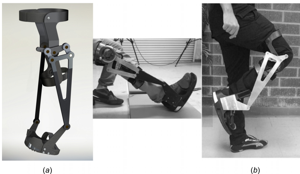
Fig. 6 (a) Computer-aided design model of prototype of KAFO device based on linkage solution 1 and (b) the corresponding manufactured prototype
