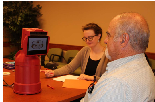
Fig. 11. Field test scene: the older adult (right), the local practitioner (middle), and the social robot (left). The clinical screening interviews are conducted by the robot and evaluated by both the robot and the independent practitioner.
