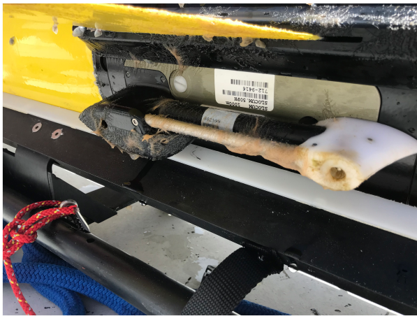
FIGURE 4 | Biofouling on the glider deep ISFET-based pH sensor after 26 days during the July–August, 2018 deployment. The glider was intercepted, cleaned, and re-deployed south of Montauk, NJ, United States on July 31, 2018.
