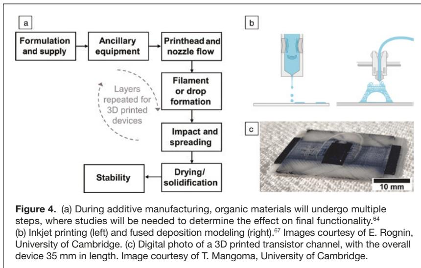
**Figure 4.** (a) During additive manufacturing, organic materials will undergo multiple steps, where studies will be needed to determine the effect on final functionality.<sup>64</sup> (b) Inkjet printing (left) and fused deposition modeling (right).<sup>67</sup> Images courtesy of E. Rognin, University of Cambridge. (c) Digital photo of a 3D printed transistor channel, with the overall device 35 mm in length. Image courtesy of T. Mangoma, University of Cambridge.
