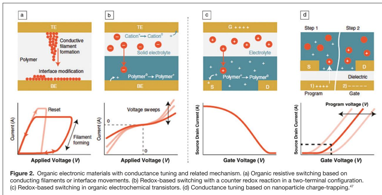
**Figure 2.** Organic electronic materials with conductance tuning and related mechanism. (a) Organic resistive switching based on conducting filaments or interface movements. (b) Redox-based switching with a counter redox reaction in a two-terminal configuration. (c) Redox-based switching in organic electrochemical transistors. (d) Conductance tuning based on nanoparticle charge-trapping.<sup>37</sup>
