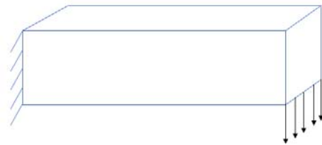
Figure 9: Loading conditions for the distributed load cantilever example problem.
