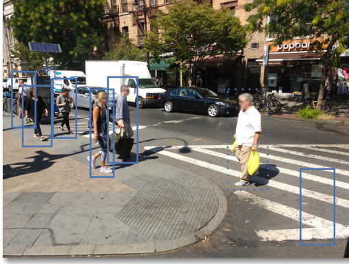
Figure 4: Hypothetical person detection. The person on the center was not identified by the detector and is a false-negative . The rightmost detection is a false-positive . Underlying image provided by Carmera.
