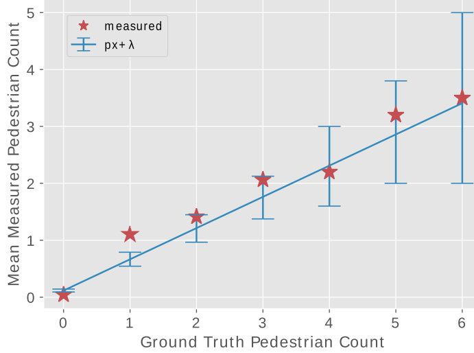
Figure 7: A comparison of the ground truth and the measured person count from the 600 tagged test images. While the actual true positive and false positive counts do not match the expected statistics (left), the total measured person count can be close to approximated as linear (right). It should be noted that this is only an approximation as, even taking sampling errors into account, the mean measured count do not fit a linear model. Error bars are the 95% confidence interval of the mean, calculated by assuming the sampling process described in Section 2.3.
