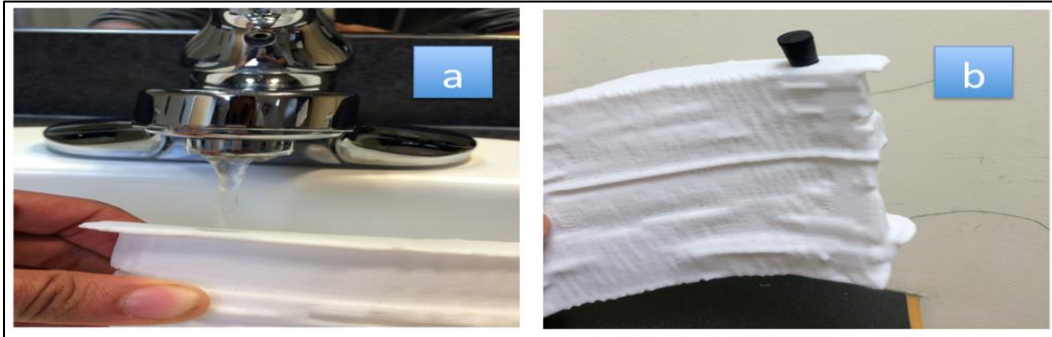
Figure 2: Testing device for leaks (a) Step 1: Device filled with water, and (b) Step 2: Hole closed with a rubber plug.
