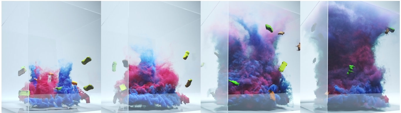
Fig. 2. Tornado. Four air inlets at the bottom of the simulation domain generate strong vortices, which quickly entangle to form a large tornado, entraining cars and cows. This two-way coupling simulation at Re=80,000 was performed on a 640 \times 720 \times 640 grid with a 4-GPU server; each frame required 139 sec.
