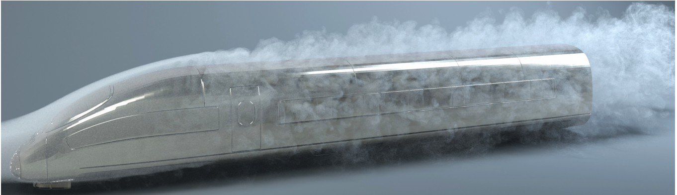
Fig. 31. Large-scale virtual wind tunnel. A static high-speed train is placed in a virtual wind tunnel (pushing air from the left); at a Reynold number of Re=28,000 and with no-slip condition inducing boundary layer turbulence, passive white particles visualize the flow separation and ensuing vortices. This simulation was computed at a resolution of 1800 \times 400 \times 400 on a 4-GPU server, each frame (i.e., 1/50 of a second) requiring 142 seconds to simulate.
