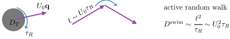
FIG. 2. Schematic of an ABP in an unbounded domain with no background flow and its long-time ( t \gg \tau_R ) active random-walk process. The swimming direction is denoted by a unit vector \mathbf{q} .
