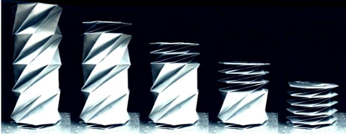
**FIGURE 1.** ORIGAMI WINE TOTE (BUILT NY, USA) CONSTRUCTED FROM MULTIPLE KRESLING LAYERS, SHOWING STABLE INTERMEDIATE CONFIGURATIONS FROM LEFT TO RIGHT AS EACH SUCCESSIVE LAYER IS COLLAPSED FROM ITS EXPANDED STATE.
