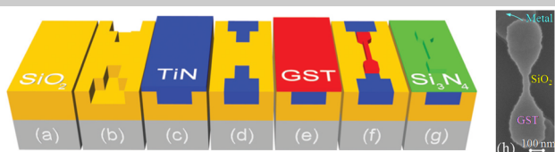
Fig. 2: Illustration of GST line cell fabrication steps (a) 700 nm \text{SiO}_2 thermal growth, (b) 250 nm deep trench formation using photolithography and reactive ion etching (RIE), (c) 300 nm TiN fill using chemical vapor deposition (CVD), (d) chemical mechanical planarization (CMP), (e) 50 nm GST film deposition by sputtering, (f) patterning of GST film using photolithography and RIE, (g) \text{Si}_3\text{N}_4 cap layer deposition, (h) SEM image of a fabricated line cell. The steps are compatible with CMOS process through back-end-of-line integration.
