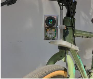
Fig. 2. The LeddarTech<sup>®</sup> Vu8 mounted on a bicycle
