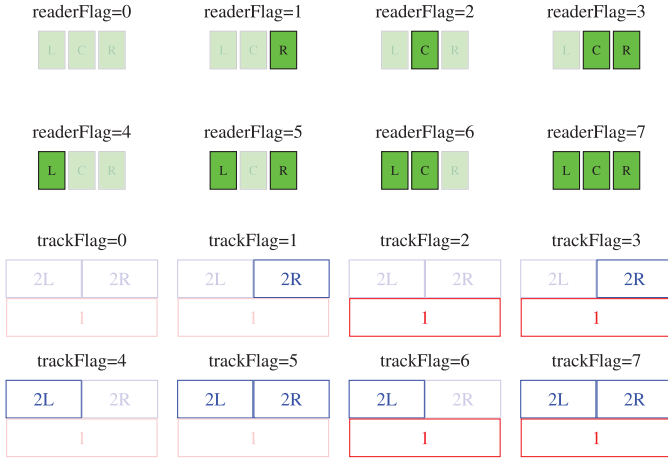
Fig. 5. Combinations of readers and tracks turned on/off for the different values of readerFlag/trackFlag.
