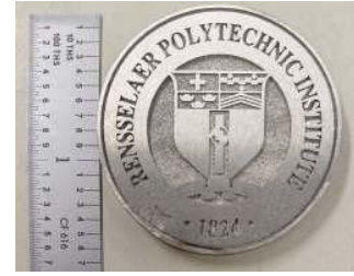
Fig. 4. A sample part produced on the SLM test bed (post-processed).
