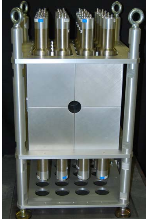
Figure 2. HECTOR: High Efficiency TOtal absorption spectrometer.
