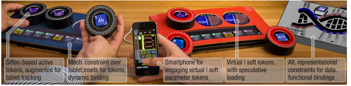
Figure 4: 2014 envisionment inset: Envisionment of Tabula prototype (one edition; inset of Figure 1). Several active tokens are present within mechanically constraining wells within physical cartouche constraints fixtured upon tablets. Two wells are physically empty, but graphically auto-filled with predictive data and tool suggestions, including a default selection. Two of the tablets (reabeled versions of working prototypes) incorporate relatively generic token constraints. A third (envisioned on right) explores more representational finger constraints for relatively persistent data, function bindings.
