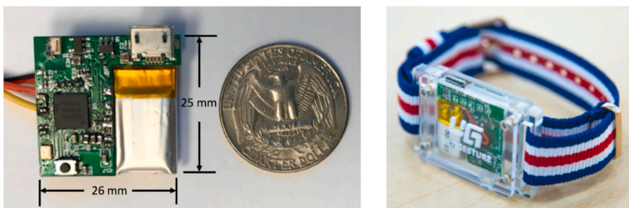
Fig. 2. UG Sensor: A combination of accelerometer, gyroscope, magnetometer.
