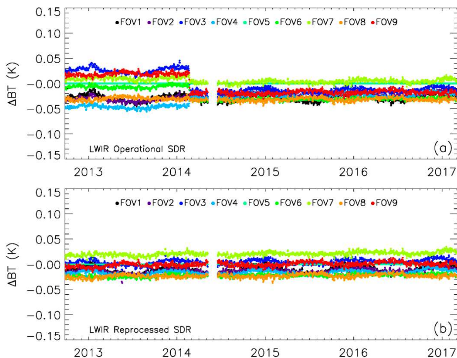
Figure 3. Time series of daily mean field of view (FOV)-to-FOV BT difference for the long-wave infrared (LWIR) band (17 channels averaged from 672 to 682\text{ cm}^{-1} ) with respect to the center FOV 5 for (a) the operational and (b) the reprocessed SDRs, respectively. The time series are for clear sky over ocean. Scan-angle-corrected SDR data from all scan angles were used in calculating the daily means. The scan-angle correction was based on Community Radiative Transfer Model (CRTM) simulations with inputs from the European Centre for Medium Range Weather Forecasts (ECMWF) analyses. The gap during the period 05/08/2014 to 06/16/2014 in the plots was caused by missing ECMWF analyses at National Oceanic and Atmospheric Administration (NOAA)/ Center for Satellite Applications and Research (STAR).
