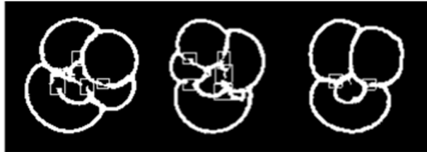
Fig. 3 Localized Topological Error Prediction. a Illustration of LTA detection used to extract bounding box used as an annotation for YOLOv3. b Examples of detection results on the training set. We can see that the first detection matches the training point shown in a . c Example of detection results on the testing set
