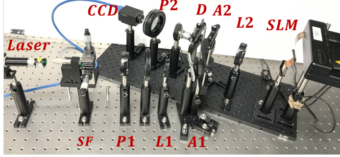
Fig. 6: Experimental setup of 3PointTM. SF : Spatial filter, L1 : collimator, L2 : Focusing lens, SLM : Spatial light modulator, P1 and P2 : Polarizers, A1 and A2 : Apertures, CCD : Sensor. The laser beam passes through SF and is collimated by L1 , and hits the reflection mode SLM, on which an input mode pattern is displayed. The modulated beam is then directed onto the diffuser D . Finally, the modulated wave is focused onto the CCD sensor.
