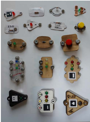
Figure 1: Multiple prototypes made with paper, cardboard, acrylic, plywood. The final prototype made with plywood was the most conductive, reliable, and reusable with magnetic terminals. However, cardboard can be used if a laser-cutter is not available in a makerspace.
